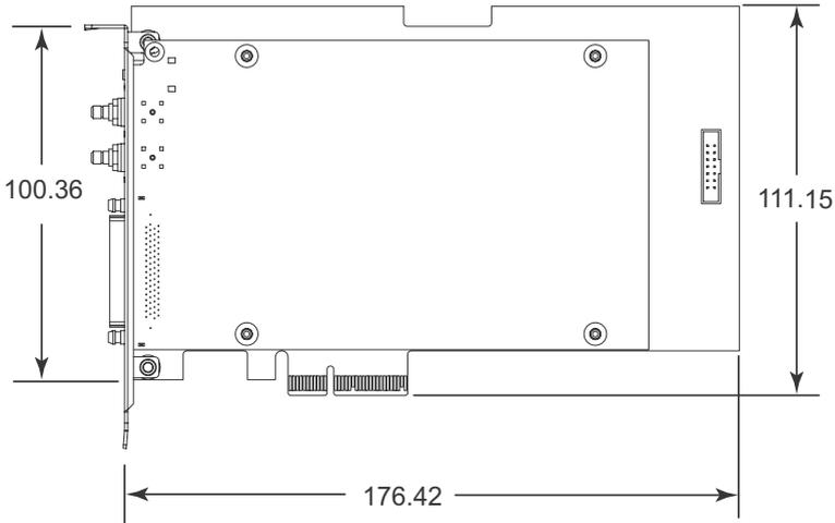
**Figure 1-3: PCIe-7360 Schematic Diagram**
