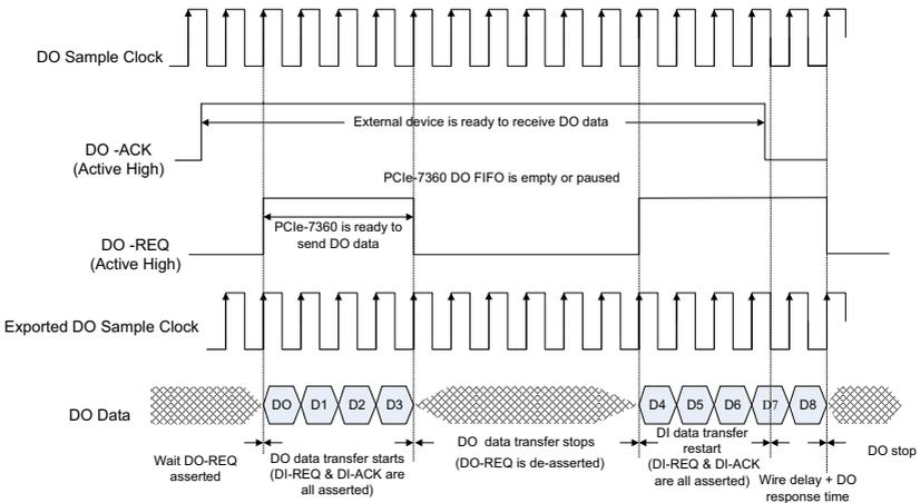
**Figure 3-22: DO Burst Handshake 2 Timing Diagram**
