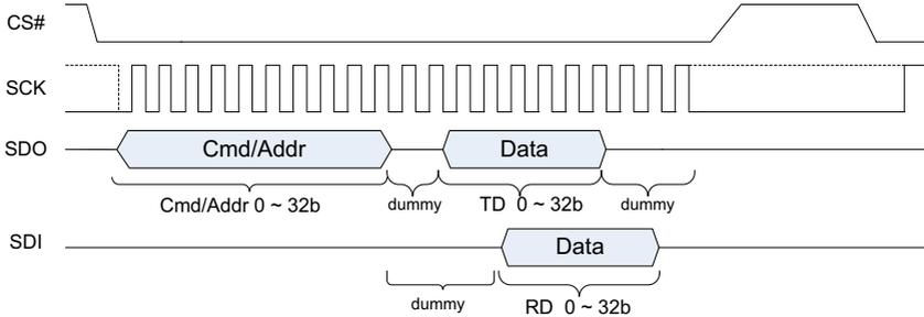
**Figure 3-33: Data Transfer on SPI Bus**
