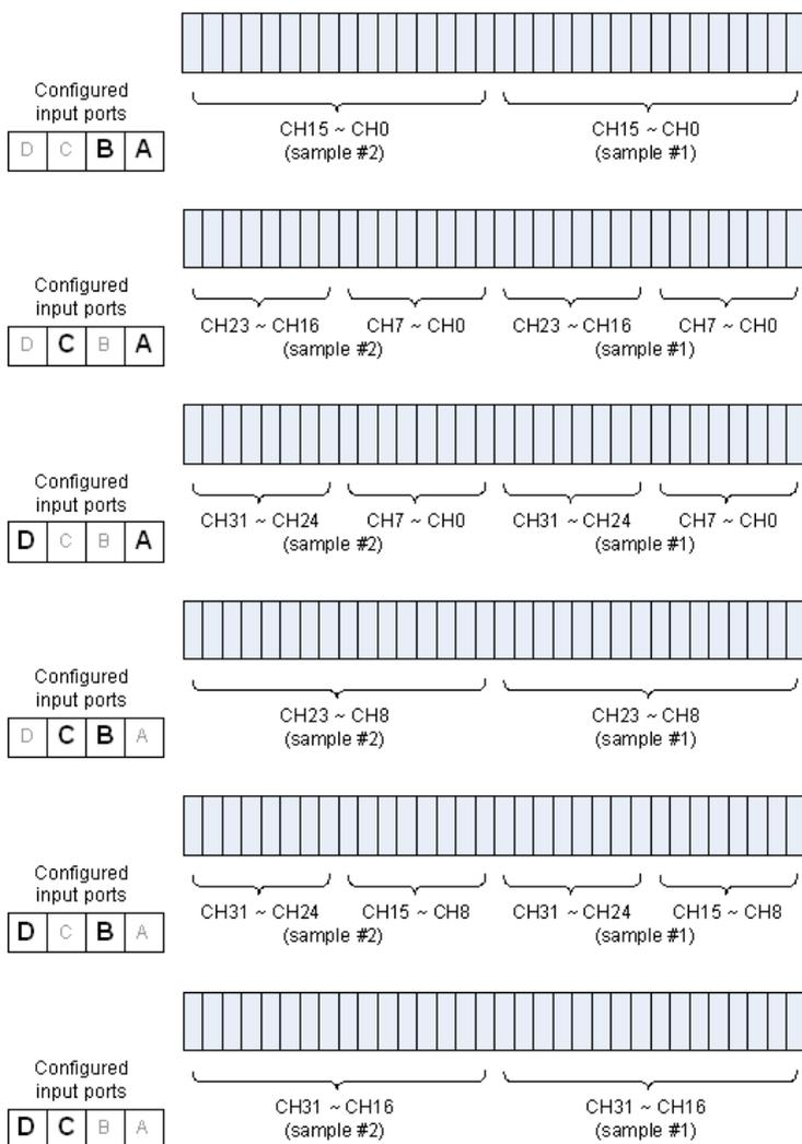
**Figure 3-3: DI raw data Mapping for 16-Bit Data Width**
