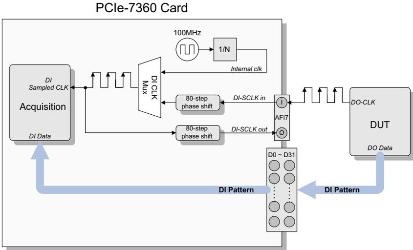
**Figure 3-39: Configured AFI7 as DI Sampled Clock In/Out**
