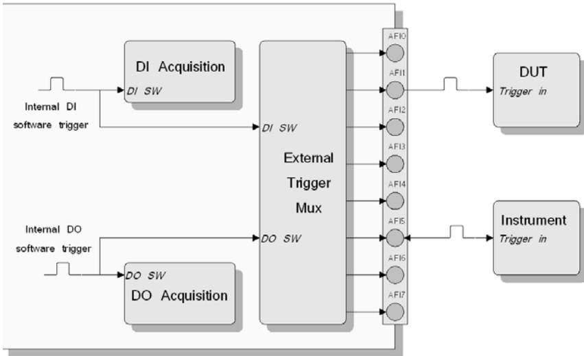
Figure 3-36: Configured AFI as Internal Software Trigger Output
