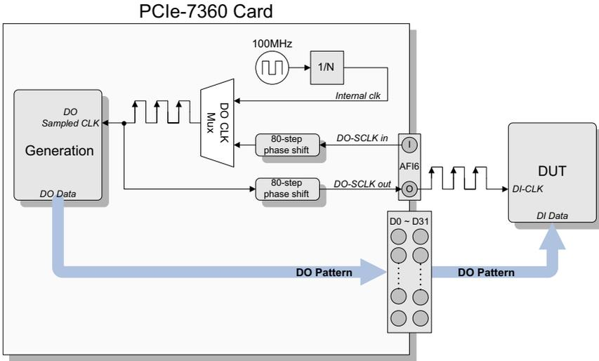
**Figure 3-40: Configured AFI6 as DO Sampled Clock In/Out**
