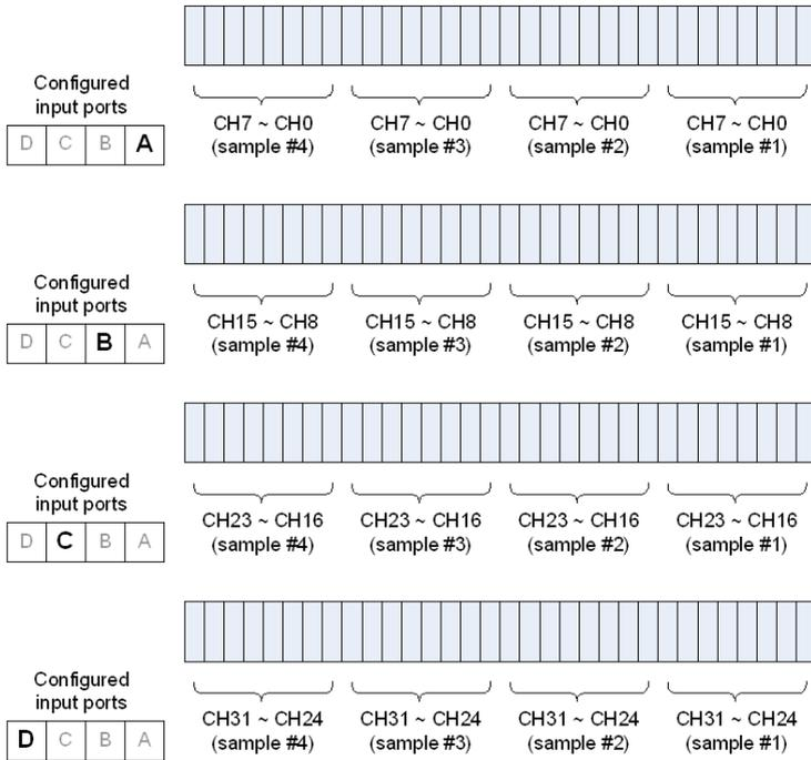
**Figure 3-2: DI Raw Data Mapping for 8-Bit Data Width**
