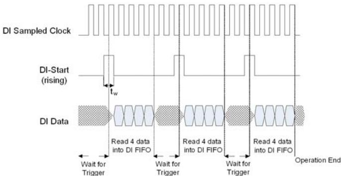
$t_w$  = Minimum required pulse width time
