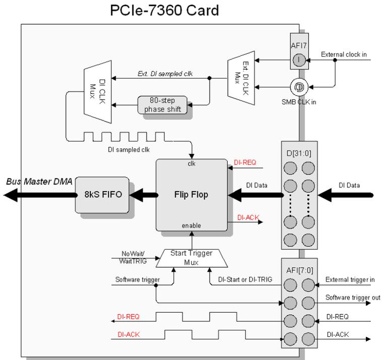
**Figure 3-18: DI Burst Handshake Mode Architecture**
