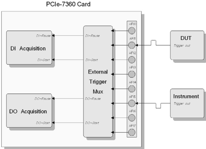
**Figure 3-35: External Digital Trigger Input Configuration**
