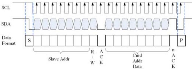
**Figure 3-30: Data Transfer on the I<sup>2</sup>C Bus**
