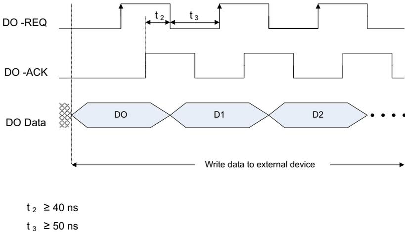
**Figure 3-17: DO Handshake Timing Diagram**
