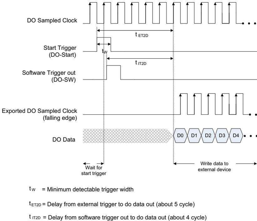
**Figure 3-13: DO Timing Diagram**
