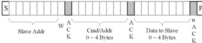
**I<sup>2</sup>C Read Command:** the format of Read command is similar with a write command except that the data part is derived by slave device.
