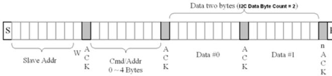
**Figure 3-31: I<sup>2</sup>C Data Format**
