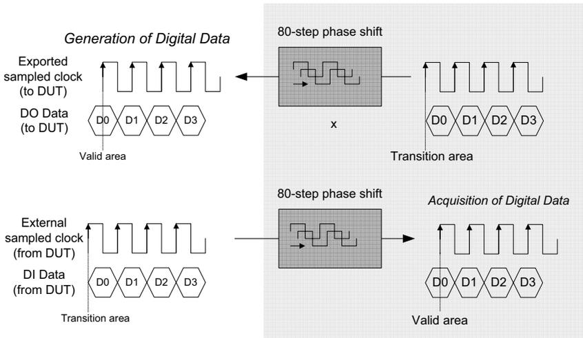
**Figure 3-6: Phase Shift of Sample Clock**
