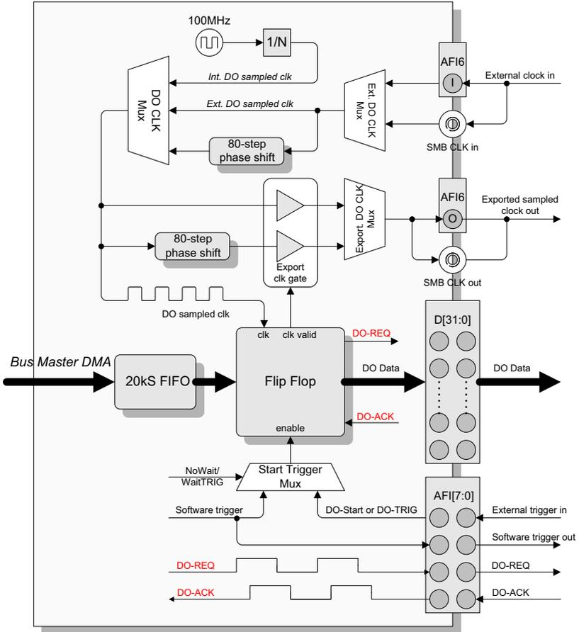
**Figure 3-20: DO Burst Handshake Mode Architecture**
