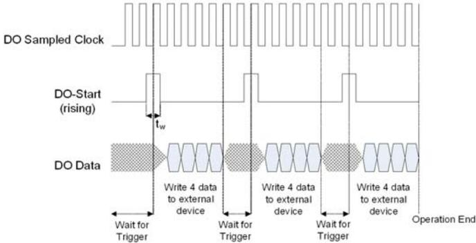
$t_w$  = Minimum required pulse width time
