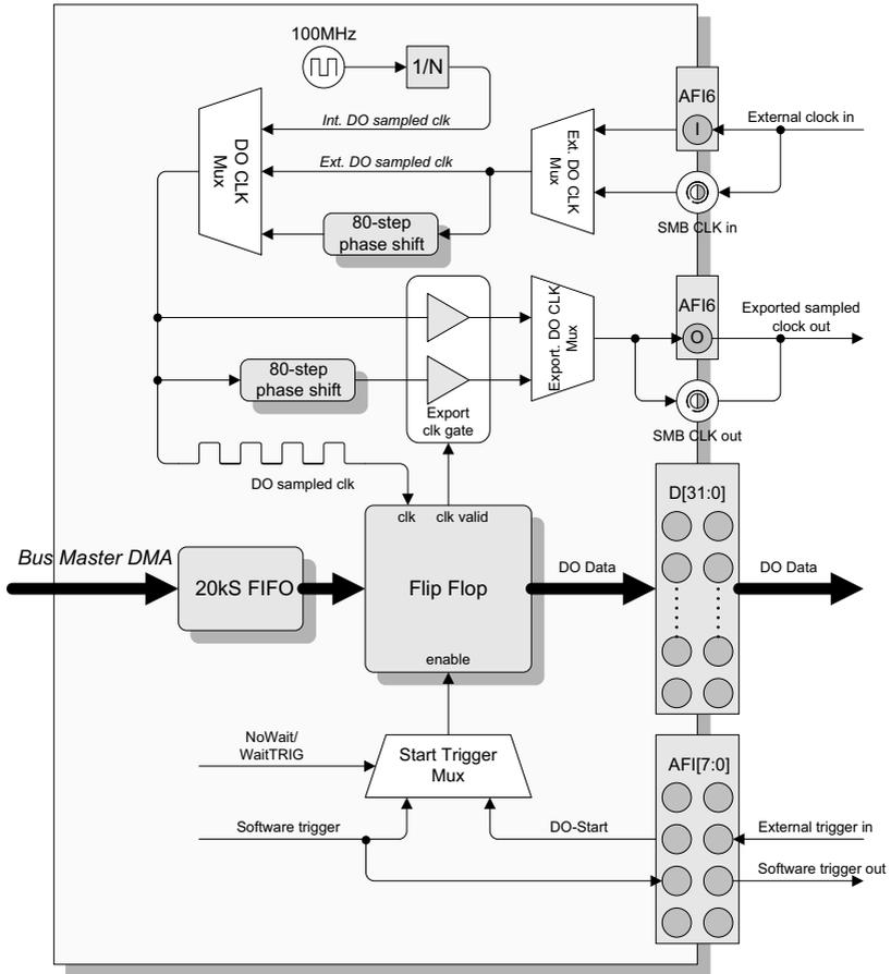
**Figure 3-12: DO Continuous Mode Architecture**
