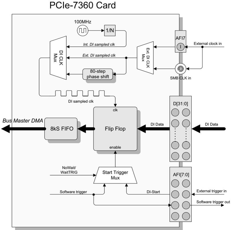
**Figure 3-10: DI Continuous Mode Architecture**
