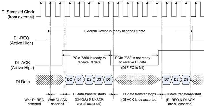
**Figure 3-19: DI Burst Handshake Timing Diagram**
