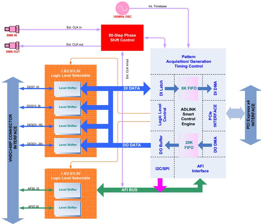
**Figure 3-1: PCIe-7360 Block Diagram**
