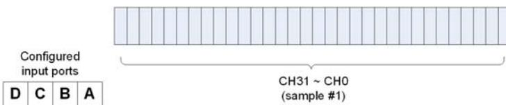
**Figure 3-5: DI raw data Mapping for 32-Bit Data Width**
