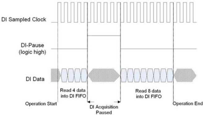
**Figure 3-27: DI Gated Trigger**
