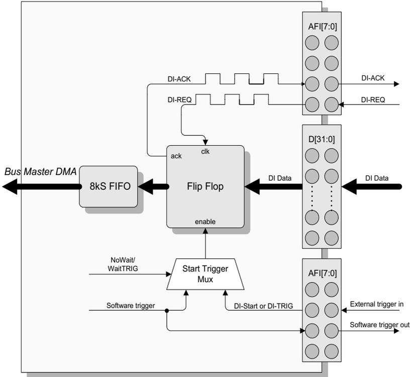
**Figure 3-14: DI Handshake Mode Architecture**
