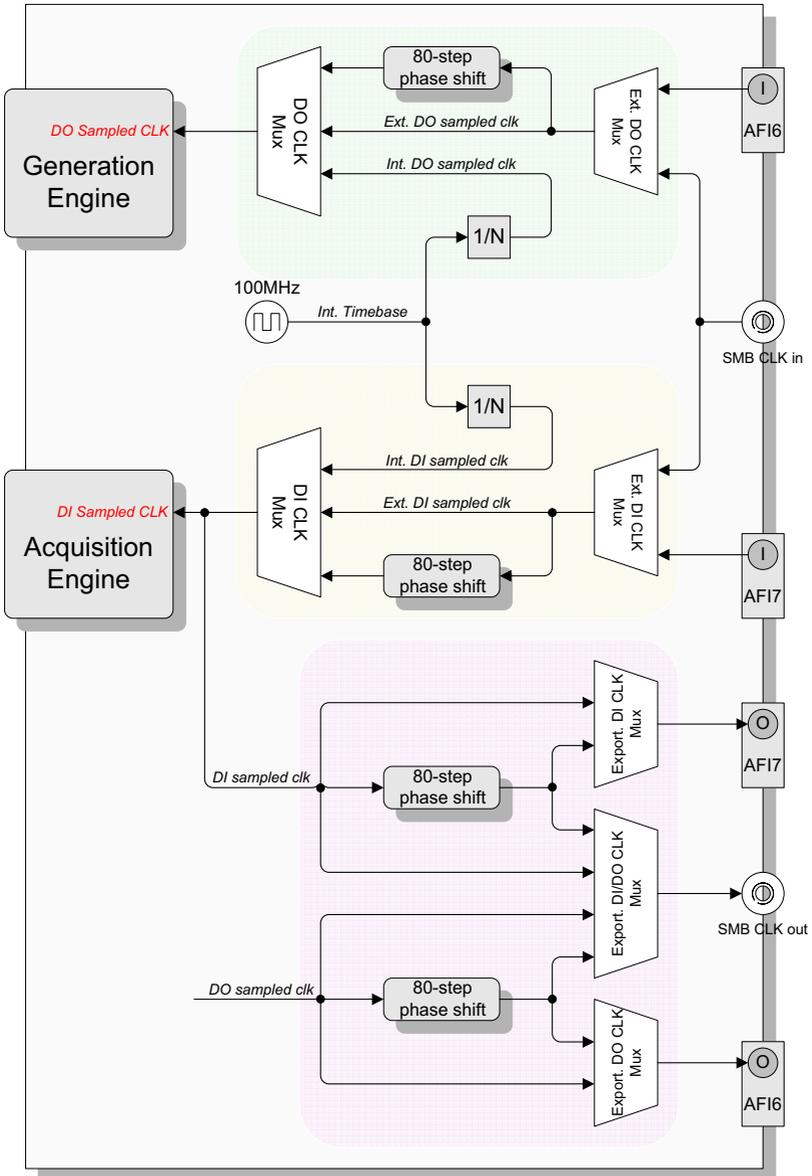
**Figure 3-9: DI/DO Sample Clock Architecture**
