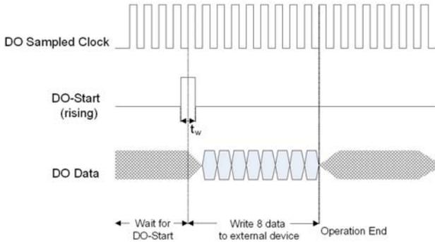
$t_w$  = Minimum required pulse width time
