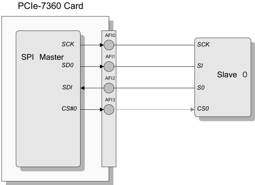
Figure 3-32: SPI Master of PCIe-7360
