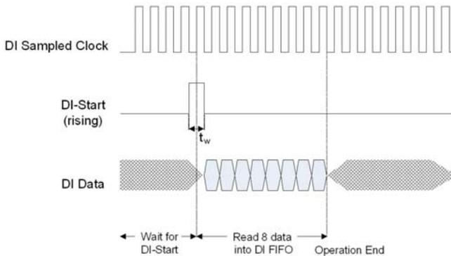
$t_w$  = Minimum required pulse width time
