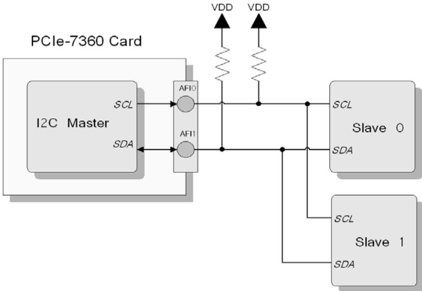
**Figure 3-29: I<sup>2</sup>C Master of PCIe-7360**
