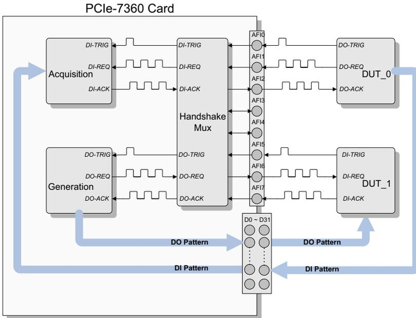
**Figure 3-38: Configured AFI as Handshake Interface**
