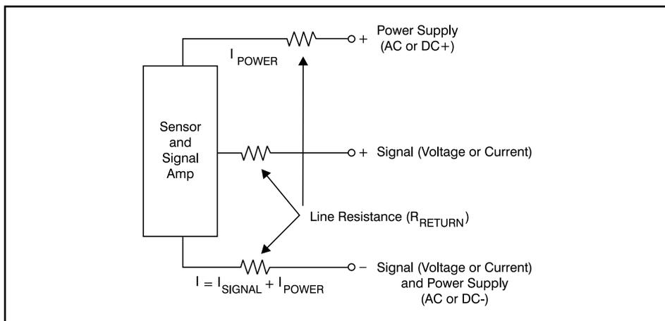
Figure 19. Three-Wire Loop
