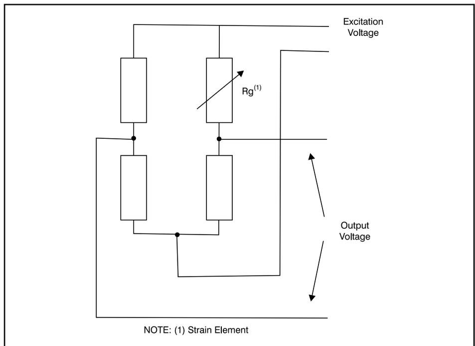
Figure 15. Quarter Bridge Strain Gage
