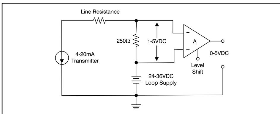
Figure 22. Typical Current Loop
