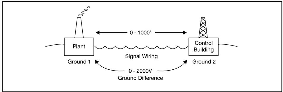
Figure 23. Differences in Ground Potential
