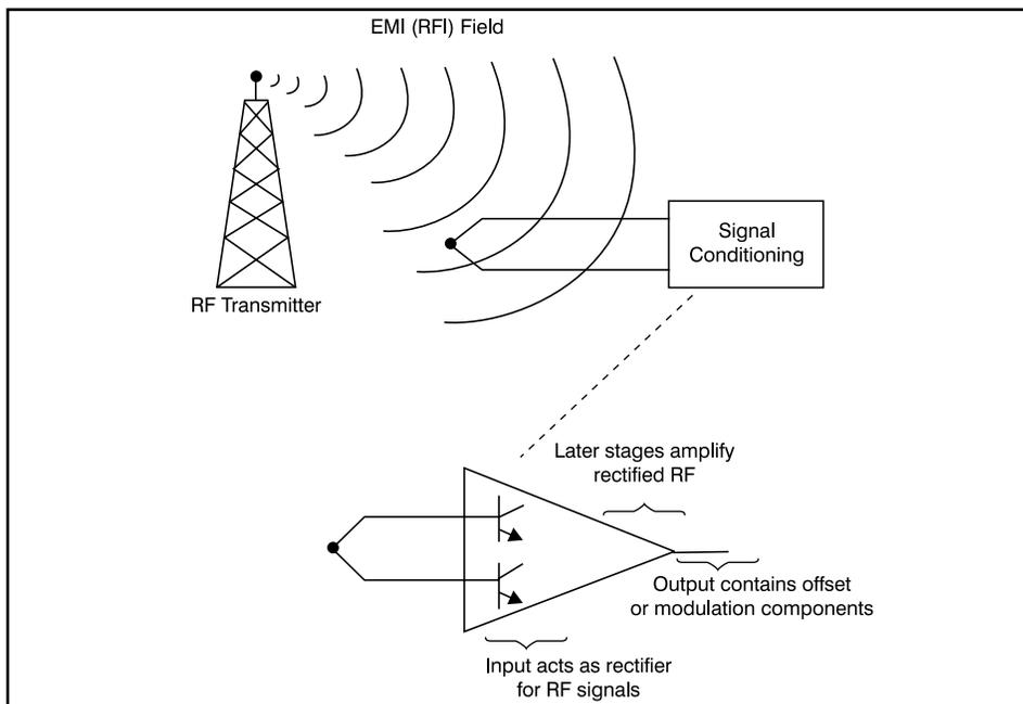
Figure 27. Electromagnetic Interference
