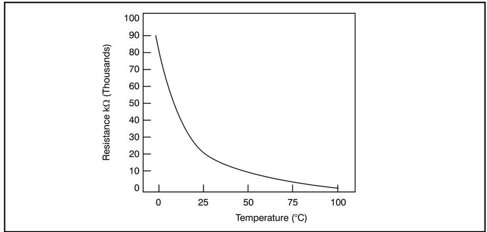
Figure 11. Typical Thermistor Characteristic
