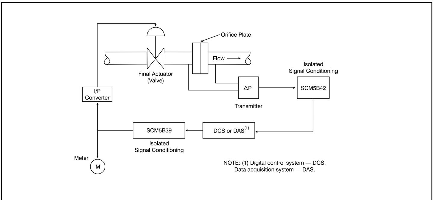
Figure 1. Typical Measurement/Control Loop
