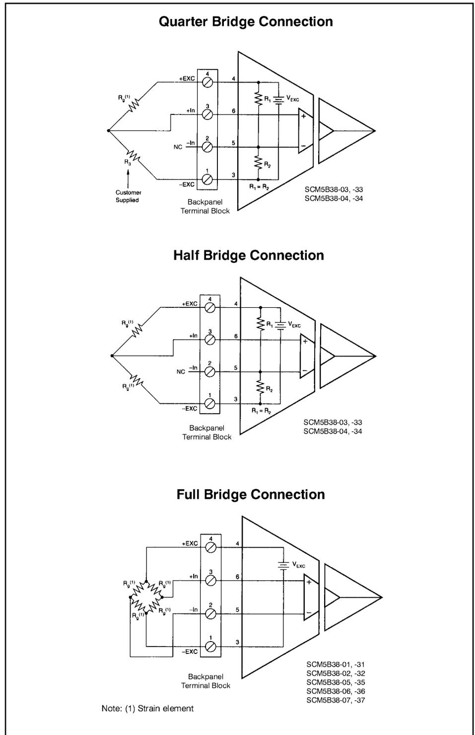
Figure 16. Strain Gage Connections to Signal Conditioning Modules (SCM5B38)
