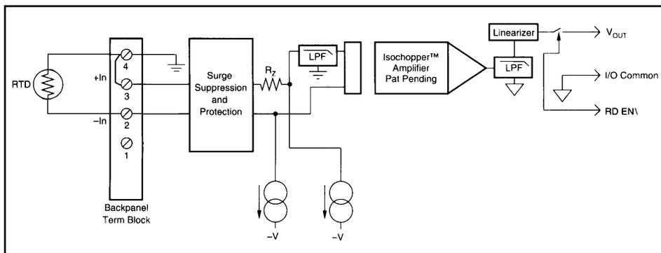
Figure 7. Two-Wire RTD Connection (SCM5B34)
