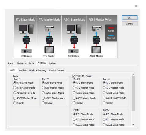
ProCOM is a Moxa proprietary function that creates virtual serial ports on the MGate MB3000 Series to make fieldbus gateway communications more versatile. This intelligent fieldbus gateway mimics the behavior of a native serial port when transmitting data to the desired destination. PCs can use ProCOM to communicate over the Ethernet with serial devices connected to the MGate MB3000 as if they were connected to the PC's
