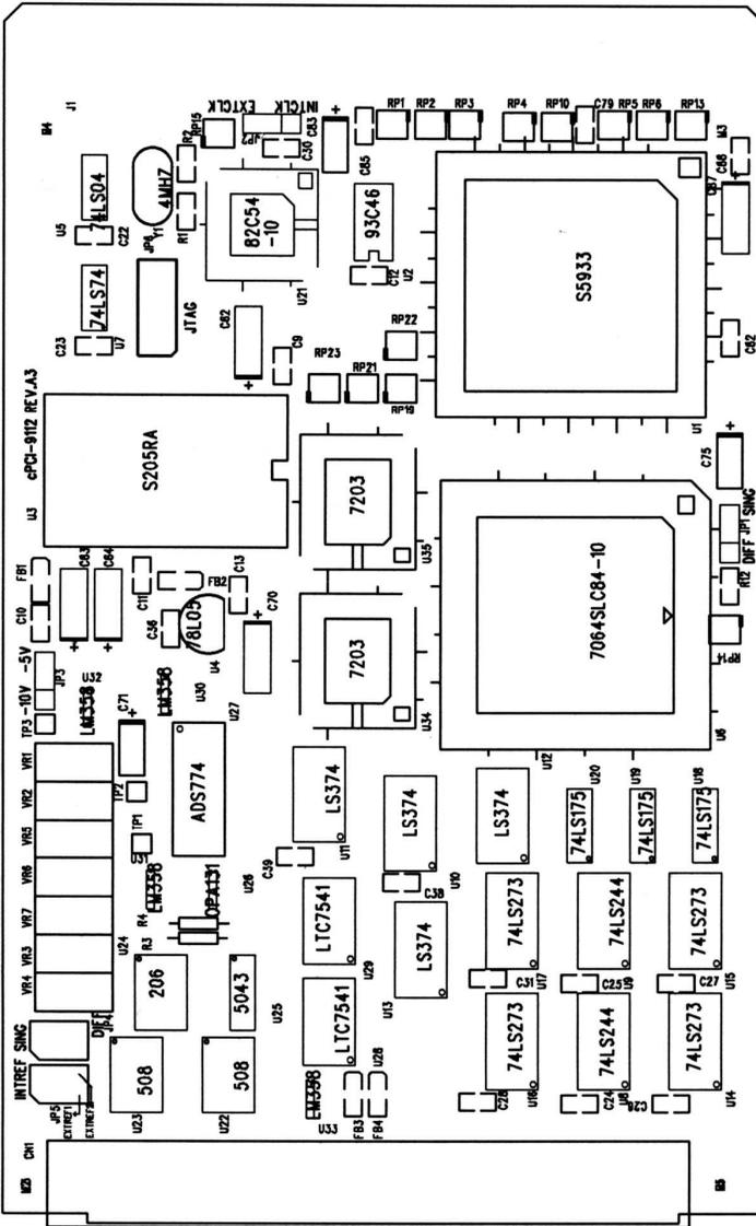
Figure 2.2 PCB Layout of the cPCI-9112
