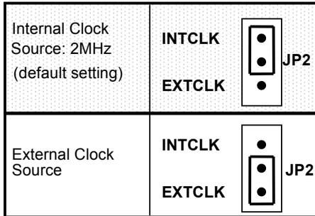
Figure 2.5 Timer's Clock Source Setting
