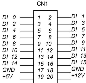
**Figure 2.8.2 Pin Assignment of CN1**
