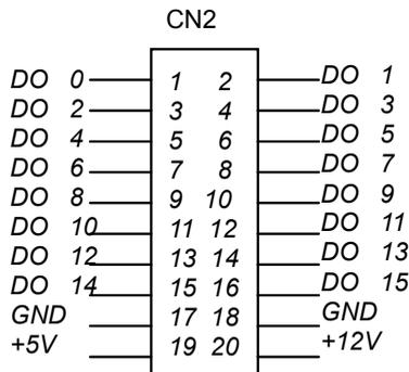
**Figure 2.8.3 Pin Assignment of CN2**
