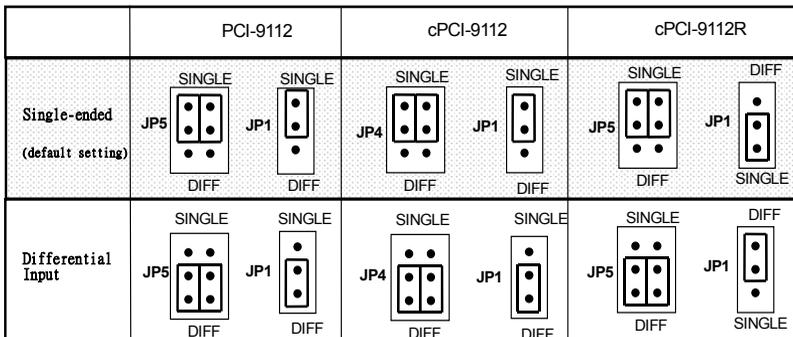
**Figure 2.4 Analog Input Mode Setting**
