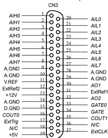
Figure 2.8.1 Pin Assignments of CN3
