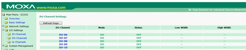
Click on a channel to see that channel's configuration options. DO Channels can operate in DO mode or Pulse Output mode. In DO mode, output is either on or off. In Pulse Output mode, a configurable square wave is generated.
