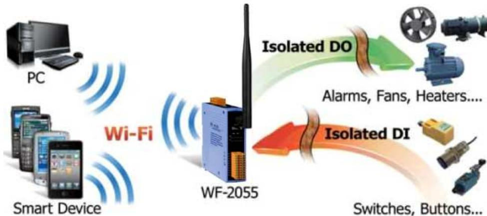
Figure 4-1: WF-2055 + PC application architecture
