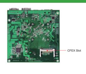
WADE-8078 is the first Portwell off-the-shelf Mini-ITX embedded board product based on the Intel® Atom™ processor E3800 product family with memory and PCI Express controller integrated to support one-channel DDR3L memory and PCI Express 2.0 lanes.Portwell has taken advantage of such technology to furnish a series of products that meets multiple industrial requirements for cost effectiveness, reliable performance and a high level of data integrity and uptime.
