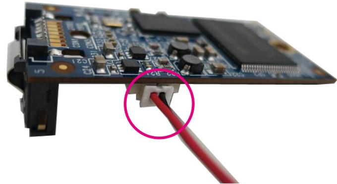
4. Install the SATA DOMM and connect the other side of SATA power cable to the SATA power connector.
