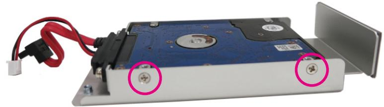
3. Connect the SATA data/power cable and fasten the cable to HDD bracket by provided screw.
