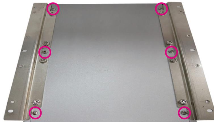
2. Lift up the cover and remove it from the chassis.
