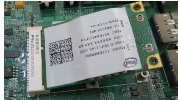
3. Push the module down and then secure it with mounting screws.
