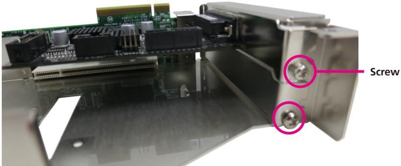
5. Secure the riser bracket to its original position.
