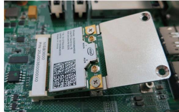
4. Push the module down and then secure it with mounting screws.
