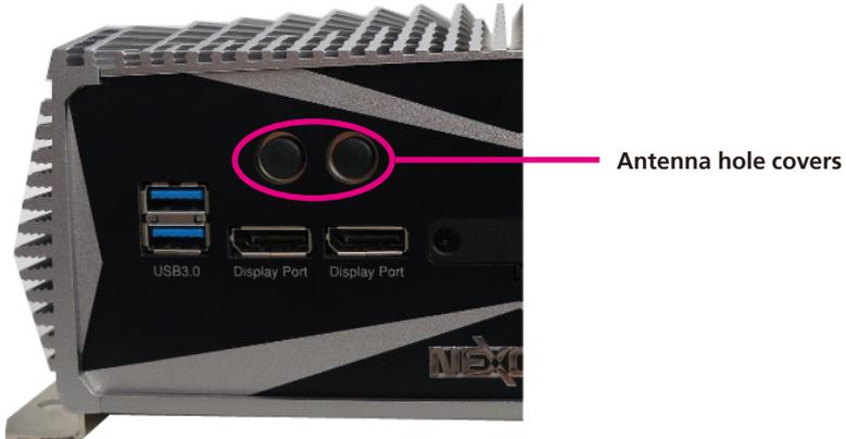
2. Insert the antenna jack through the antenna hole.
