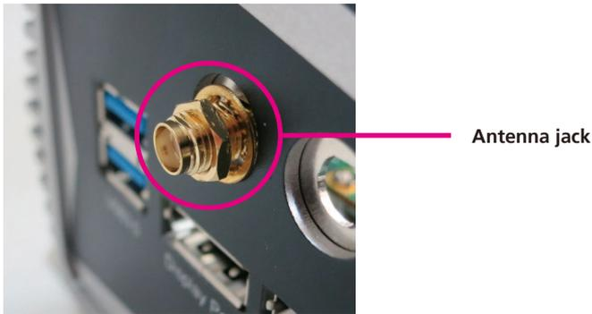
3. Insert the 2 rings (ring 1 and ring2) onto the antenna jack.
