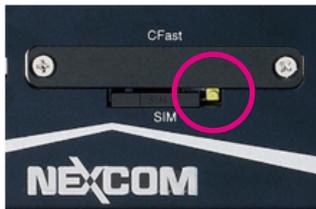
3. Place the SIM card to the SIM card holder and secure it to the original position.
