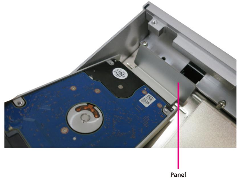
5. Connect the SATA data/power cable to the connector on the SATA drive then secure the HDD bracket to its original place.
