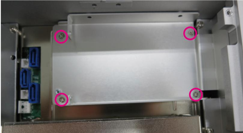
2. Use the provided screws to secure the drive in place.
