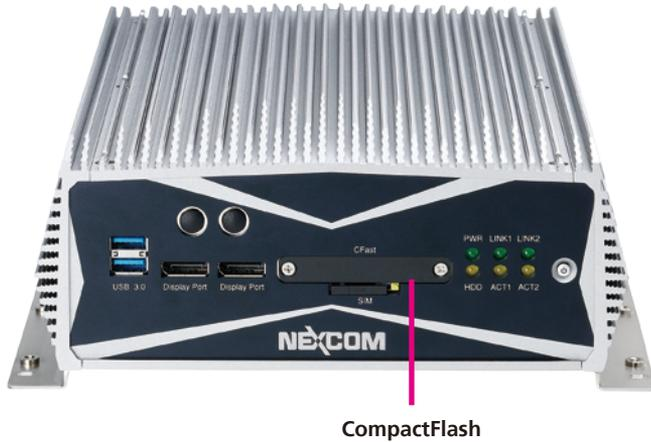
2. Remove the mounting screws and cover of the CompactFlash socket.
