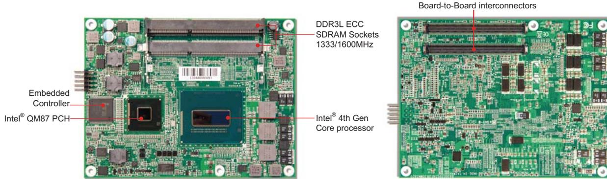
PCOM-B630VG can offer high computing power by Shark Bay processor brings quad core technology and provides significant performance improvement. 6GT/s SATA performance is supported by PCOM-B630VG. It supports storage back-up function and enhances performance ability. We also provide SOL, IDER, Serial over Lan and Remote control functions in PCOM-B630VG by Intel® iAMT 9.0 support.
