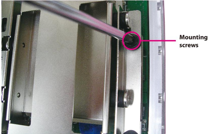
8. With both the hard drive bays installed, secure them together by tightening screws into the center where the two brackets meet.
