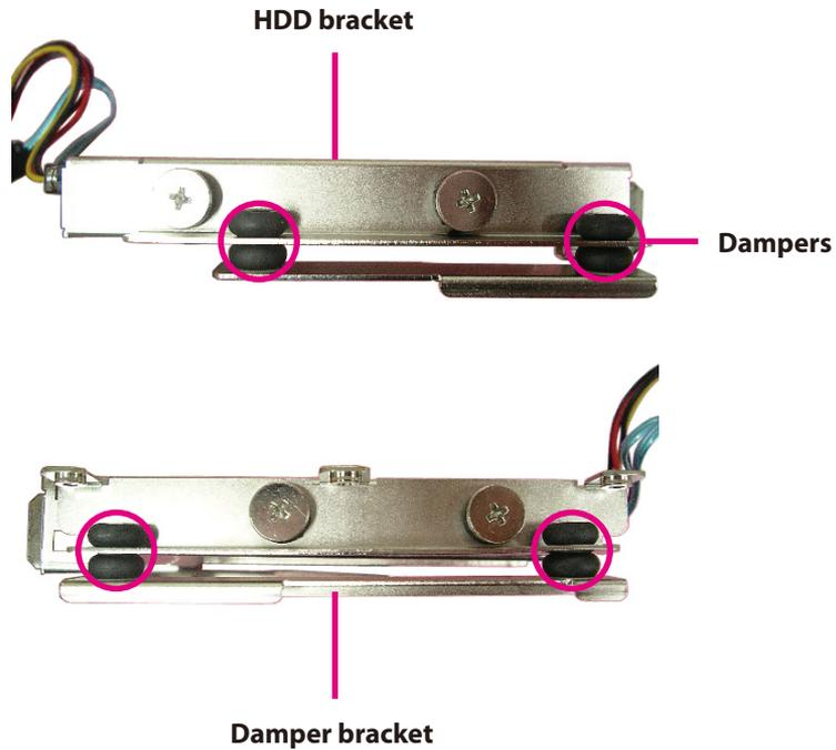
6. With the damper brackets secured, install the left hard drive bracket onto the left side of the motherboard and secure the bracket using screws.
