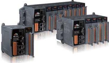
WinPAC-8000 is the new generation PAC of ICP DAS. It is equipped a PXA270 CPU (520 MHz) running a Windows CE.NET 5.0 operating system, various connectivities (VGA, USB, Ethernet, RS-232/485) and 1/4/8 slots for high performance Parallel I/O modules (high profile I-8K series) and serial I/O modules (high profile I-87K I/O modules).
